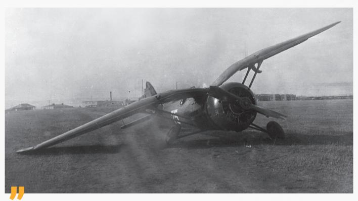
Final photo in the series, this one allows a good view on the leading edge colour demarcation line. Worth noting are the wing machine gun covers made of canvas, which proves that it was possible to fly with them put on. (Dan Antoniu/Horia Stoica collection)
