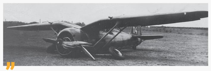
One more shot from the front. Note the faintly visible underwing cockade and again the glossy look of the airplane, making the reconstruction of camouflage a very time-consuming task. Well visible is the way in which wooden propellers shatter on impact. (Dan Antoniu/Horia Stoica collection)
